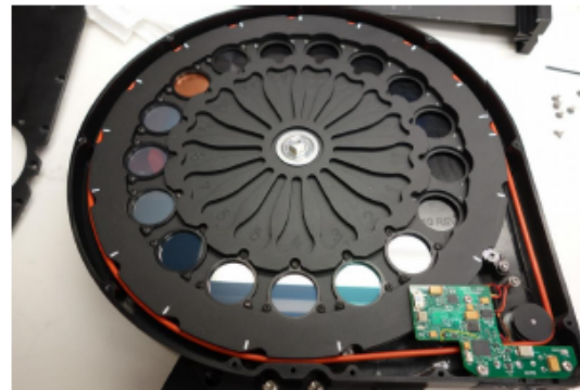
Filter wheel to explore the range 8-50 \mu\text{m}
